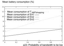
Figure 3: Battery consumption vs probability of bandwidth to be *low*.
