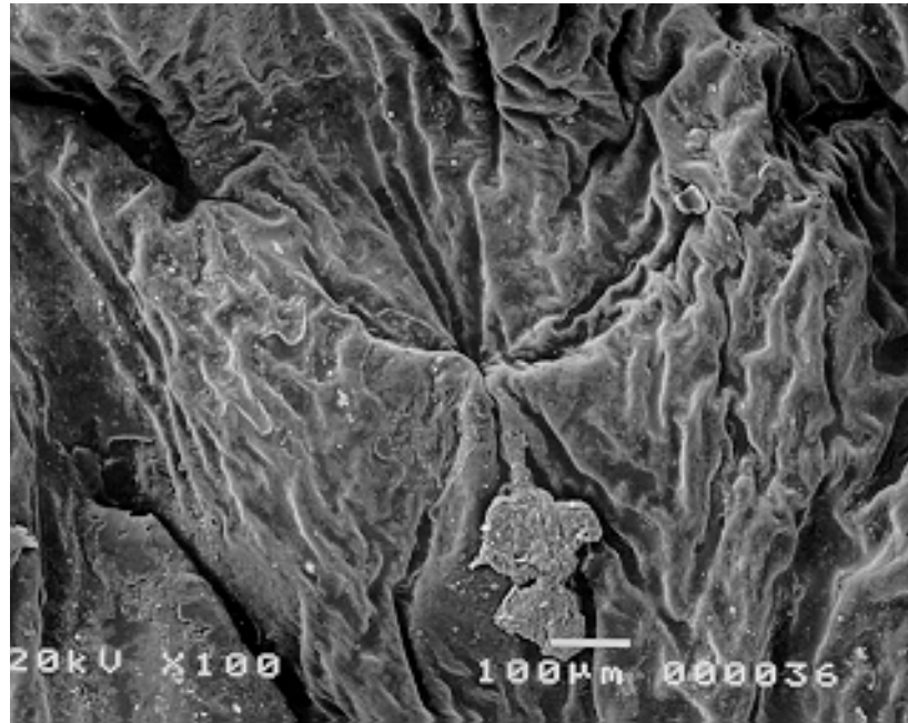
Figure 11. Electron micrograph of flavedo side after D.I.C preprocessing at 5.8 bar, 50 % initial moisture content and a processing time of 3 minutes.
