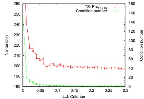
Fig. 3. Influence of the poor quality elements on the condition number for the thermal simulation.
