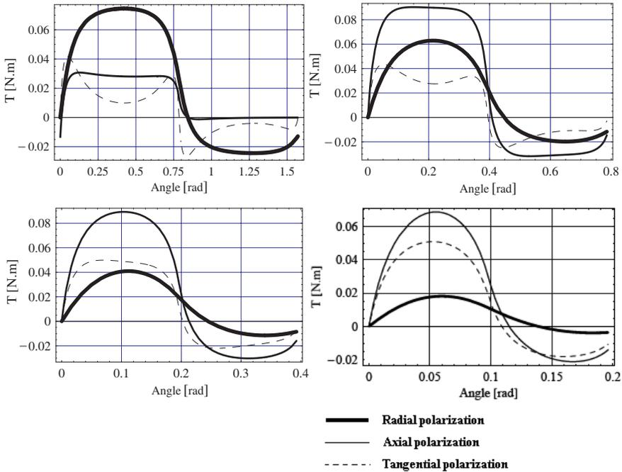
**Figure 8.** Representation of the torque transmitted between two rotors with a plane air gap with tile permanent magnets radially, tangentially and axially magnetized. The angular widths taken are  $\frac{\pi}{4}$  rad,  $\frac{\pi}{8}$  rad,  $\frac{\pi}{16}$  rad and  $\frac{\pi}{32}$  rad respectively from the upper figure to the lower figure.
