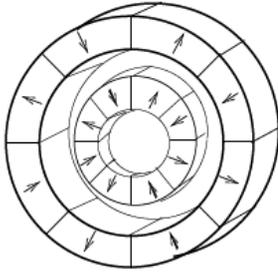
**Figure 1.** Magnetic coupling using a cylindrical air gap and tile permanent magnets radially magnetized.
