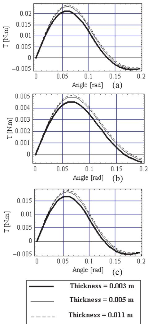
**Figure 10.** Representation of the torque transmitted between two rotors with a cylindrical air gap with tile permanent magnets radially (a), axially (b) and tangentially (c) magnetized with three magnet thicknesses (0.003 m, 0.005 m, 0.011 m); we take the following dimensions:  $r_2 = 0.024$  m,  $r_3 = 0.025$  m,  $z_1 = 0$  m,  $z_2 = 0.003$  m,  $z_3 = 0$  m,  $z_4 = 0.003$  m,  $J_1 = J_2 = 1$  T,  $\theta_4 - \theta_3 = \theta_2 - \theta_1 = \frac{\pi}{32}$ .
