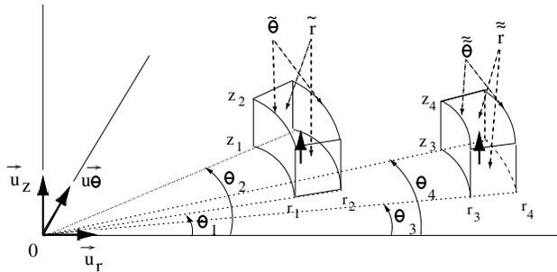
Figure 6. Two tile permanent magnets axially magnetized.
