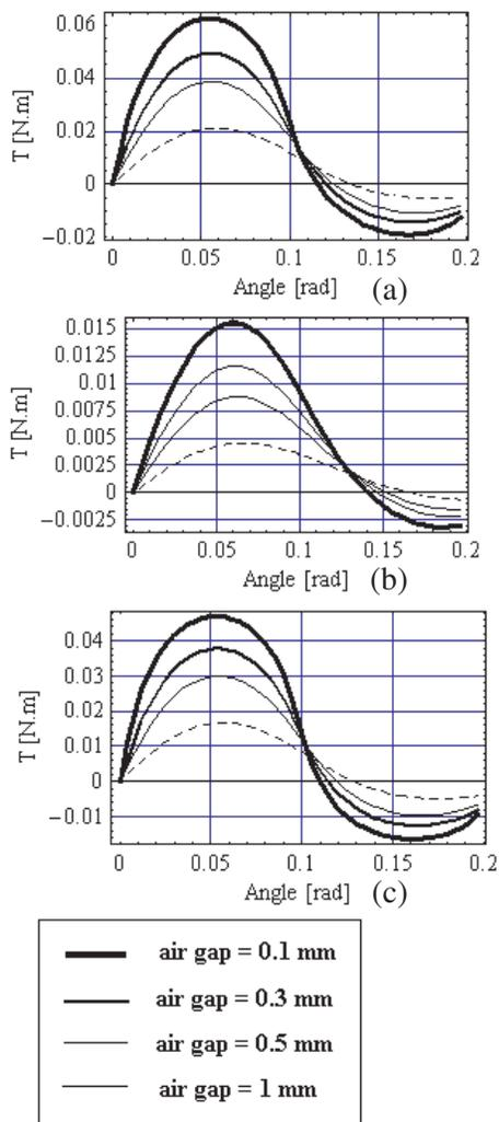
**Figure 9.** Representation of the torque transmitted between two rotors with a cylindrical air gap with tile permanent magnets radially (a) axially (b) and tangentially (c) magnetized with four air gaps (0.1 mm, 0.3 mm, 0.5 mm, 1 mm); we take the following dimensions:  $r_2 - r_1 = 0.003$  m,  $r_4 - r_3 = 0.003$  m,  $z_1 = 0$  m,  $z_2 = 0.003$  m,  $z_3 = 0$  m,  $z_4 = 0.003$  m,  $J_1 = J_2 = 1$  T,  $\theta_4 - \theta_3 = \theta_2 - \theta_1 = \frac{\pi}{32}$ .
