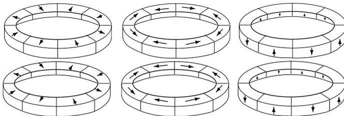
**Figure 4.** Magnetic couplings using plane air gaps; from left to right: coupling using tile permanent magnets radially magnetized, coupling using tile permanent magnets tangentially magnetized, coupling using tile permanent magnets axially magnetized.
