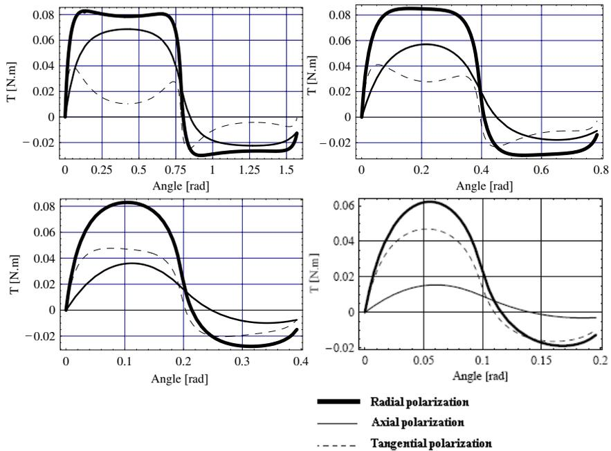
**Figure 7.** Representation of the torque transmitted between two rotors with a cylindrical air gap with tile permanent magnets radially, tangentially and axially magnetized. The angular widths taken are  $\frac{\pi}{4}$  rad,  $\frac{\pi}{8}$  rad,  $\frac{\pi}{16}$  rad and  $\frac{\pi}{32}$  rad respectively from the upper figure to the lower figure.
