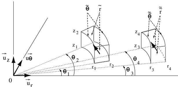
**Figure 5.** Two tile permanent magnets tangentially magnetized.
