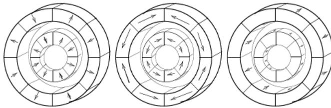
**Figure 3.** Magnetic couplings using cylindrical air gaps; from left to right: coupling using tile permanent magnets radially magnetized, coupling using tile permanent magnets tangentially magnetized, coupling using tile permanent magnets axially magnetized.
