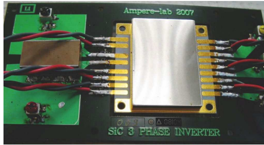
Figure 3: A JFET-based, 540 V, 15 A, 3-phase inverter (6 JFETs) in a single package with an external DC capacitor. This system has been successfully tested at 200°C.
