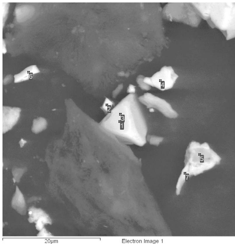
Fig. 9. SEM backscattering image of magnetic grains extracted from sample K228, Kafan section.
