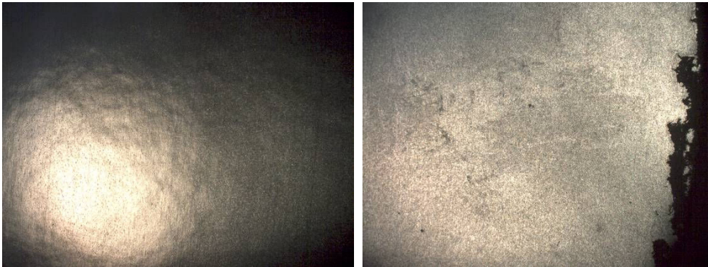
Figure 10a) Ti layer before electroplating tin and Figure 10b) Ti layer after electroplating tin
