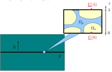
Figure 3: Macroscopic fracture interpreted as a porous medium  $(\Omega_F = \Omega_s \bigcup \Omega_p)$
