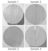
Figure 1: Photograph of various samples after Brazilian splitting test, which shows the variability in the initial fracture: (a) concrete samples; (b): Callovo-Oxfordian argillite.
