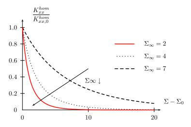
Figure 8: Effect of  $\Sigma_{\infty}$  on the normalized permeability evolution,  $\phi_0 = 0.5$ )
