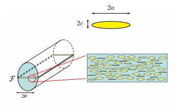
Figure 4: The fracture modelled as a distribution of discrete parallel cylinders
