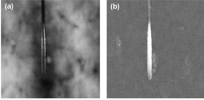
FIG. 2. Typical AFM height (a) and phase (b) images of the crack tip for a fracture propagating from top to bottom of the image ( $1 \times 1 \mu\text{m}$ ). The linear gray scale range is, respectively, 10 nm and  $10^\circ$ .
