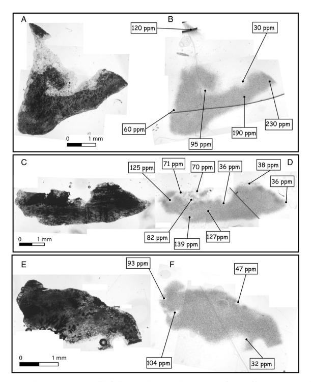
Fig. 7. Same as Figs. 5 and 6. TM90 17, crocodilian fossil osteoderm (TM90, Late Miocene). A, C and E: fragments of the same tooth. B, D and F: induced fission tracks images of these fragments on the external detector after irradiation.
