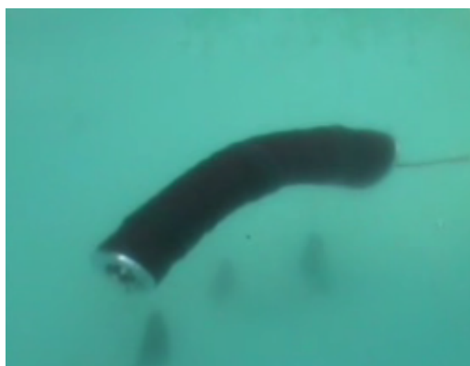
Figure 17. PICTURE OF A 6 VERTEBRAE IN A SWIMMING POOL TO TEST THE WATERTIGHTNESS AND BUOYANCY
