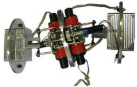
Figure 8. PROTOTYPE OF TWO VERTEBRAE MADE BY TECHNICAL STAFF OF THE IRCCyN
