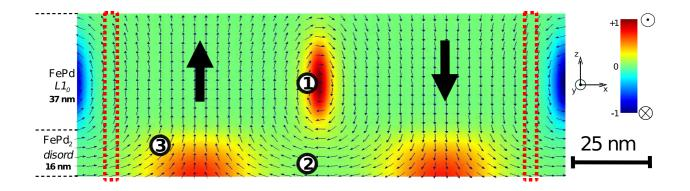
Figure 1: Micromagnetic simulation from GL\_FFT on the FePd bi-layer. The input parameters are displayed in the text. The simulations contain only the magnetic layers. The growth direction is along the vertical. A colour scale is used for the component of magnetization perpendicular to the figure. Marks on the figure show the in-plane magnetic components described in the text. Dashed areas correspond to some areas which fulfil the no-deflection conditions.
