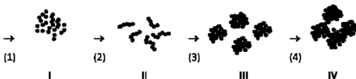
Fig 1: Representation of the steps of a 4-scale agglomeration according to Refs. [8] and [9]
