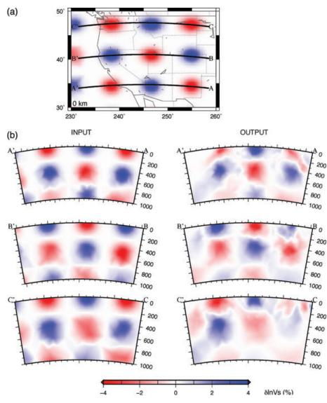
**Figure B3.** (a) Map view showing the locations of the cross-sections. (b) Vertical resolution for  $\delta \ln V_S$ . The input anomalies are equally spaced balls, in which the anomaly amplitude decays with increasing radius following a Gaussian curve. The 1/e width of the Gaussian curve is 300 km.
