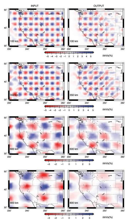
**Figure B1.** Lateral resolution for  $\delta \ln V_S$ . The depth of each map is indicated at the lower left-hand corner. The input anomalies are equally spaced balls, in which the anomaly amplitude decays with increasing radius following a Gaussian curve. At 100 and 350 km depths, the 1/e width of the Gaussian curve is 150 km. At 600 and 800 km depths, the 1/e width of the Gaussian curve is 300 km.
