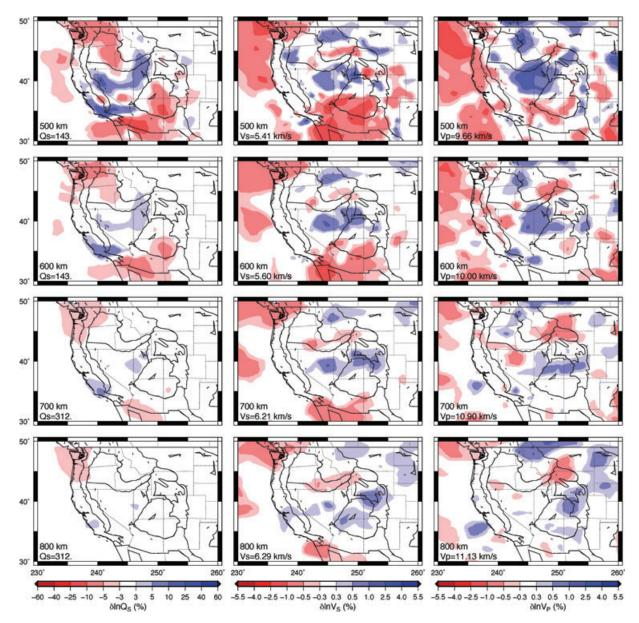
**Figure A2.** Map views of the preferred models of  $\delta \ln Q_S$  (left-hand panel) and  $\delta \ln V_S$  (centre panel), and the  $\delta \ln V_P$  model (right-hand panel) by Sigloch *et al.* (2008), at 500, 600, 700 and 800 km depths in the western US. Geological and political boundaries are plotted. Depth and the reference model value are shown at the lower left-hand corner of each map.
