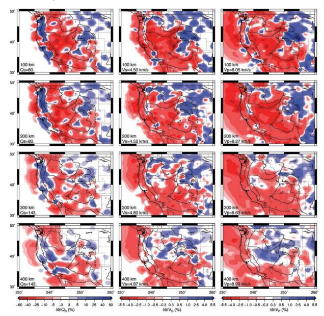
**Figure A1.** Map views of the preferred models of  $\delta \ln Q_S$  (left-hand panel) and  $\delta \ln V_S$  (centre panel), and the  $\delta \ln V_P$  model (right-hand panel) by Sigloch *et al.* (2008), at 100, 200, 300 and 400 km depths in the western US. Geological and political boundaries are plotted. Depth and the reference model value are shown at the lower left-hand corner of each map.
