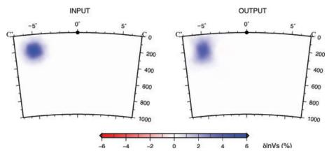
**Figure B4.** Resolution test of the 'slab hole'. The input model is a ball in which the anomaly amplitude decays with increasing radius following a Gaussian curve. The 1/e width of the Gaussian curve is 200 km. The ball is centred at (45.2°N, 238°E) and at 200 km depth, approximately the same location as the 'slab hole' shown in Fig. 10 section CC'. The cross-section is the same as the cross-section CC' in Figs 9(a) and 10.
