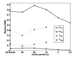
**Figure 12.** The relative weight of  $\delta \ln V_S$  and  $\delta \ln Q_S$  in contributing to the data fit. It is measured as the rms ratio of the predictions relative to the observations. The observations are  $\delta T$  in the case of  $c_{\text{TV}}$ ,  $c_{\text{TQ}}$  and  $\delta \ln A$  in the case of  $c_{\text{AV}}$ ,  $c_{\text{AO}}$  (see eq. 5).
