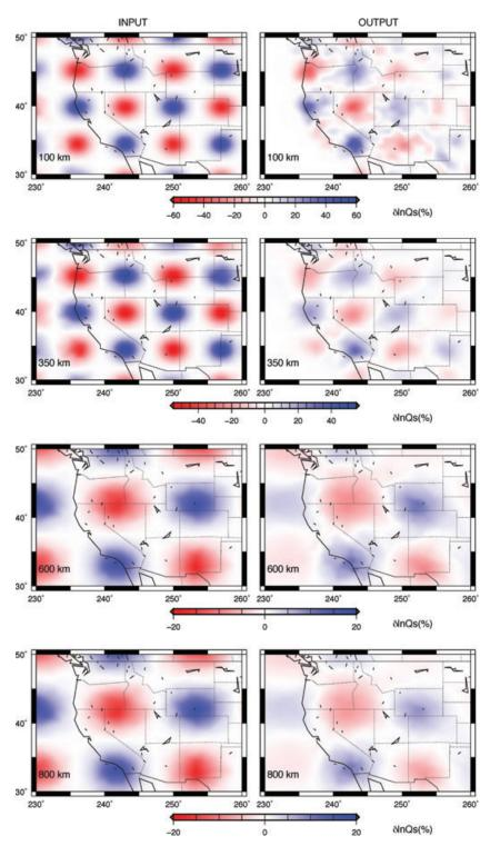
**Figure B2.** Lateral resolution for  $\delta \ln Q_S$ . The depth of each map is indicated at the lower left-hand corner. The input anomalies are equally spaced balls, in which the anomaly amplitude decays with increasing radius following a Gaussian curve. At 100 and 350 km depths, the 1/e width of the Gaussian curve is 300 km. At 600 and 800 km depths, the 1/e width of the Gaussian curve is 500 km.
