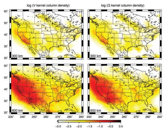
**Figure 7.** Sensitivity of the model parameters  $V_S$  and  $Q_S$  to the data. The maps show the logarithm (base 10) of the kernel column density (eq. 3) for  $V_S$  and  $Q_S$  at 300 km and 600 km depths, with the absolute level of max<sub>j</sub>  $\sum_i K_{ij} = 4381$  s for the  $V_S$  kernel and max<sub>j</sub>  $\sum_i K_{ij} = 552$  for the  $Q_S$  kernel. Zero means maximum density.
