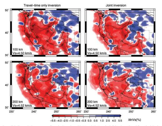
**Figure 14.** Comparison of shallow velocity structures from the inversion with  $\delta T$  and  $\delta \ln V_S$  only (left-hand panel) and from the joint inversion (right-hand panel). Geological and political boundaries are plotted. Depth and the reference model value are shown at the lower left-hand corner of each map.
