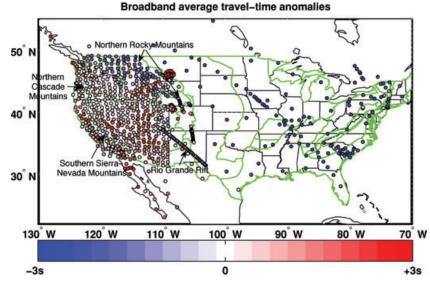
Figure 5. Broad-band traveltime anomalies averaged at each station. Positive values reflect slow velocity anomalies in the vicinity of the station, and negative values indicate fast velocity anomalies. Examples of local structures expressed by traveltimes anomalies are labelled. Green lines delineate the geological boundaries in the US.
