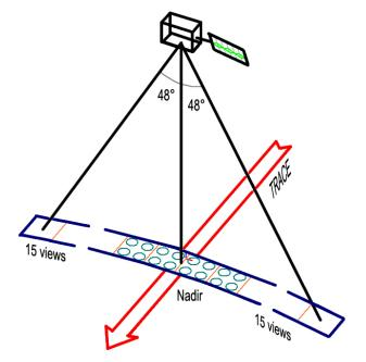
Fig. 1. IASI observing mode: the instrument measures the spectrum of infrared radiation emitted by the Earth and the atmosphere, from a low altitude sun-synchronous orbit, over a swath width of  $\sim$ 2200 km, every 50 km at nadir (with 4 footprints of 12 km in diameter).
