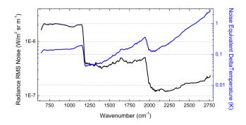
**Fig. 2.** IASI radiometric noise as established from a set of representative spectra, spanning a range of latitude. Values are provided in radiance units ( $W/(m^2 \text{ sr m}^{-1})$ , black line, left scale), and were converted to noise equivalent temperature difference (Ne $\Delta T$ , blue line, right scale) for a given reference temperature of 280 K.
