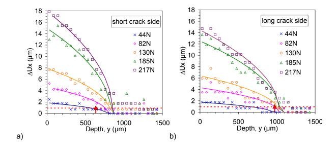
Figure 8 : Change with load of the crack opening displacement profile along crack depth (a) on the short and (b) long crack side; the dashed-line corresponds to 3 times the uncertainty in  $U_x$  and the arrow indicates the position of the crack front plotted in Figure 7. The solid lines correspond to the best fitting curves.
