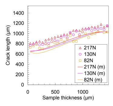
Figure 10: Crack tip position of the equivalent "elastic crack" based on the SIF extractor method (symbols); the solid lines correspond to the crack tip positions reported in Figure 5b (visual inspection of tomographic images and smoothed by curve fitting).
