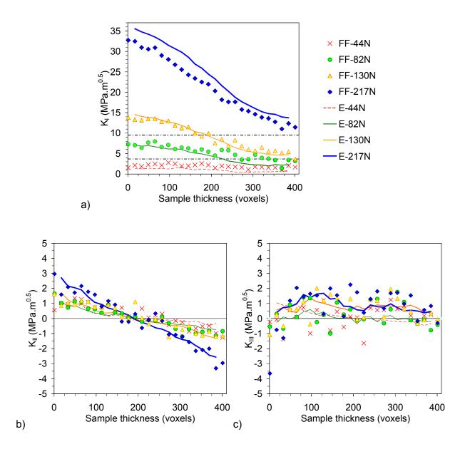
Figure 9 : SIF values along the crack front for (a) Mode I, (b) Mode II and (c) Mode III; Measured ('FF') values of SIF (symbols) are compared to computed ('E') values (lines); the hatched area in (a) corresponds to the  $K_{op}$  range obtained from literature data.
