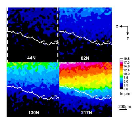
Figure 7: Maps of  $\Delta U_x$  displacement (COD) in the specimen cross-section with increasing load. The crack front is drawn in white and the dashed-lines along y direction indicate the location of the profiles plotted in Figure 8.
