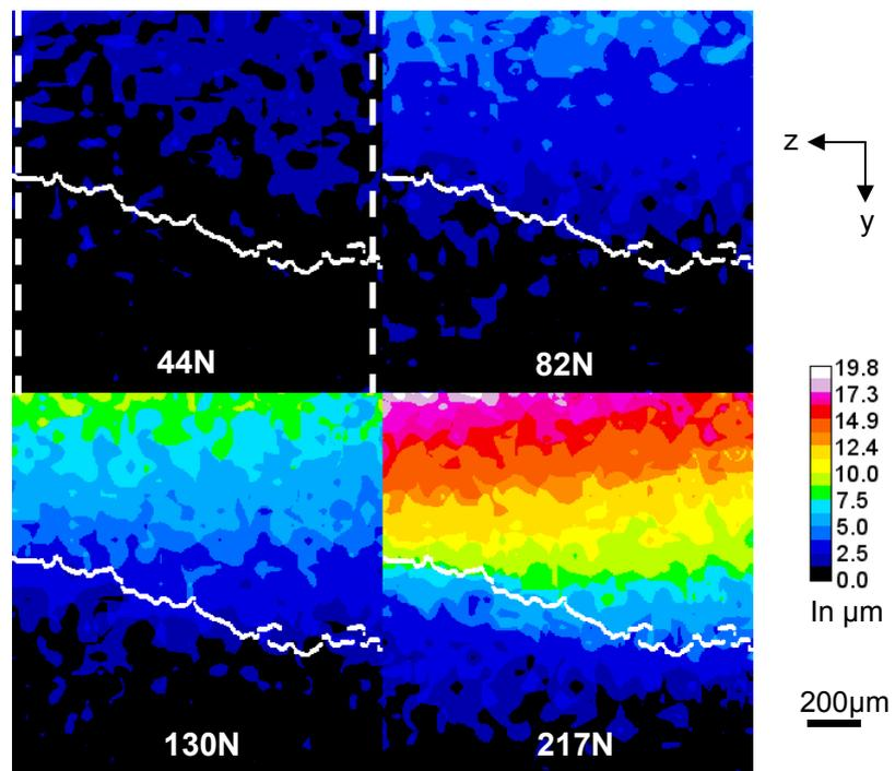
Figure 7 : Maps of  $\Delta U_x$  displacement (COD) in the specimen cross-section with increasing load. The crack front is drawn in white and the dashed-lines along  $y$  direction indicate the location of the profiles plotted in Figure 8.
