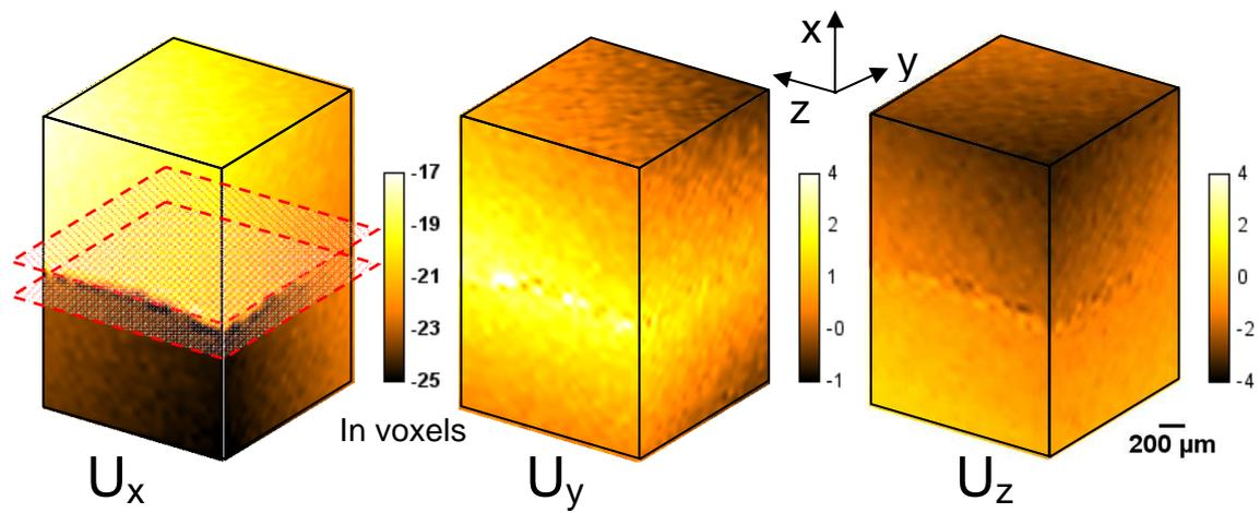
Figure 6 : Displacement (expressed in voxels) fields in the specimen volume under maximum load (macroscopic load applied along  $x$  direction). The hatched planes drawn in the  $U_x$  field indicate the  $(y, z)$  planes used for COD mapping in Figure 7.
