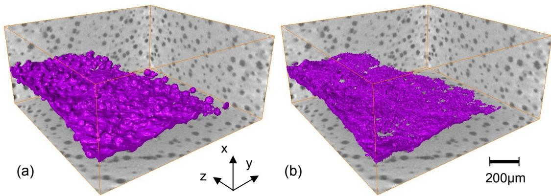
**Figure 4 : 3D rendering of the crack surface at maximum load from (a) the thresholded tomographic image and from (b) the residual error field.**
