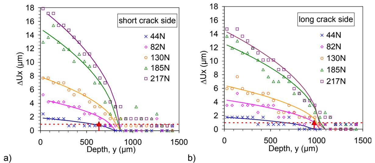
**Figure 8 : Change with load of the crack opening displacement profile along crack depth (a) on the short and (b) long crack side; the dashed-line corresponds to 3 times the uncertainty in  $U_x$  and the arrow indicates the position of the crack front plotted in Figure 7. The solid lines correspond to the best fitting curves.**
