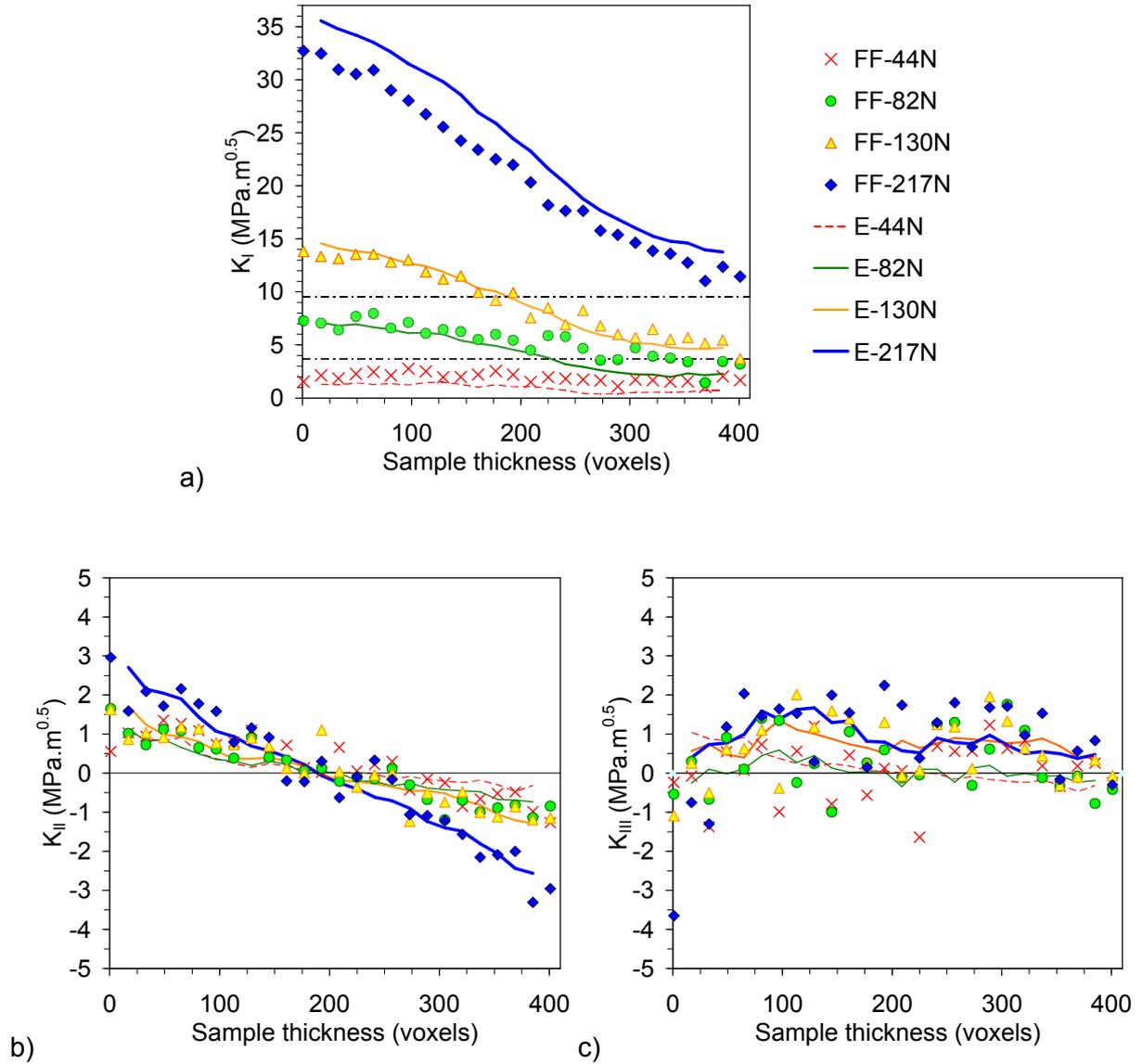
**Figure 9 : SIF values along the crack front for (a) Mode I, (b) Mode II and (c) Mode III; Measured ('FF') values of SIF (symbols) are compared to computed ('E') values (lines); the hatched area in (a) corresponds to the  $K_{op}$  range obtained from literature data.**
