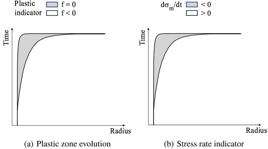
Fig. 4. Space-time diagram for a hollow sphere (initial outer radius:  $b = 12.5 \mu\text{m}$ , initial inner radius  $a = 0.58 \mu\text{m}$ ) submitted to a stress rate of  $2 \text{ GPa}/\mu\text{s}$  on the outer radius. The material parameters are those of tantalum (Table 1). The plastic zone coincides with the region in which the local pressure decreases, in spite of an overall pressure increase.
