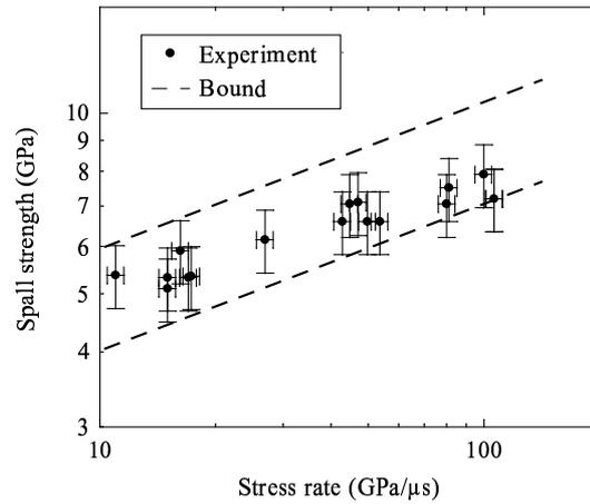
Fig. 12. Spall strength vs. stress rate for tantalum. The solid symbols are experimental points and the dashed lines are the bounds built from Eqs. (33) and (34) with  $\alpha = 1/2$ , and  $m = 8$  determined from Fig. 10.
