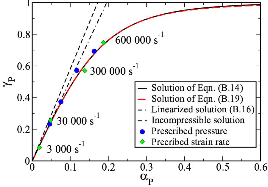
Fig. B.1. Dimensionless velocity  $\gamma_P = \dot{c}/c_P$  of the plastic zone vs. dimensionless growth velocity  $\alpha_P = \dot{a}/c_P$  of a cavity in a compressible and incompressible medium (the value of  $c_P$  at finite compressibility is used for all curves). Material parameters of tantalum (Table 1), except for the bulk modulus in the incompressible case.
