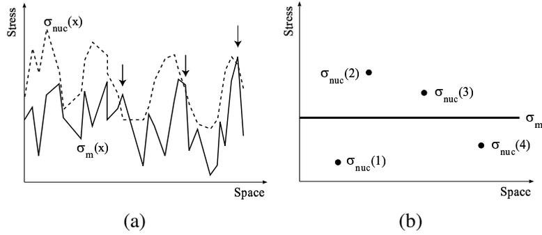
Fig. 2. Simplifying assumptions of the nucleation model (nucleation conditions met at arrows). a) Physical situation: applied tensile stress  $\sigma_m$  and nucleation level  $\sigma_{nuc}$  as continuous random fields. b) Simplification: uniform applied stress, and field of nucleation thresholds split up into discrete sites of random locations and threshold values.
