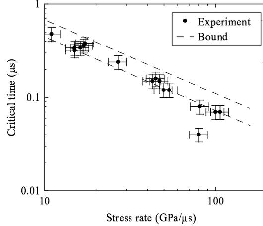
Fig. 11. Critical time vs. stress rate. The solid symbols are experimental points and the dashed lines are the “bounds” built from Eqn. (33) with  $\alpha = 1/2$ , and  $m = 8$  determined from Fig. 10.
