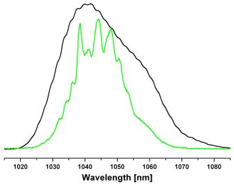
Figure S2: The spectrum of the Yb-amplifier frequency comb (black), smoothed over 50 points, incident on the optical cavity. The spectrum transmitted from the cavity when the comb frequencies are locked to the cavity modes (green).
