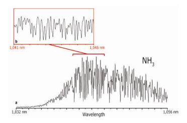
Figure 4. Cavity-enhanced spectrum of the crowded region of the  $3v_1$  overtone band of ammonia. The cavity is filled with 50 hPa of ammonia. The weak transitions are observed at high resolution for the first time to our knowledge and are of interest for the modeling of radiative transfer in the atmospheres of the giant Jovian planets.
