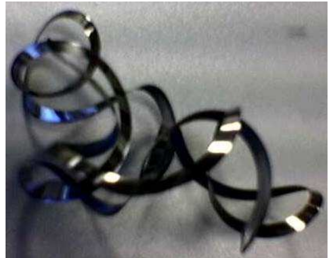
Fig. 8 Chip related to a_p = 3 mm, f = 0.1 mm/rev and the spindle speed N = 690 rpm
