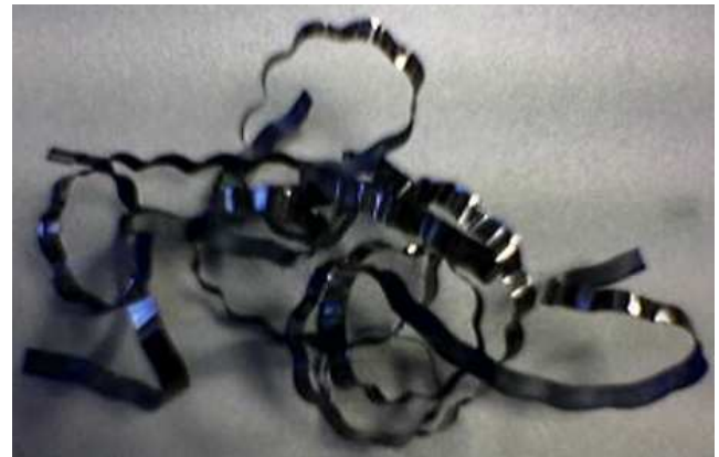
Fig. 9 Chip related to a_p = 4 mm, f = 0.1 mm/rev, and the spindle speed N = 690 rpm.
