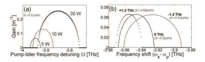
Fig. 2. (a) MI gain versus sideband MI frequency detuning for different input pump powers and  $\Delta\omega=0.$  (b) MI gain versus ( $\omega_s$ - $\omega_p$ ) for different frequency separations  $\Delta\omega$  and P=5 W.
