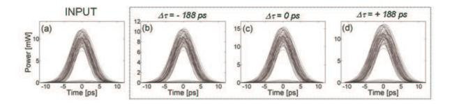
Fig. 5. Eye diagrams for a 40-Gbit/s PRBS signal. Pulse train (a) after propagation through a transmission line, at the delay generator output for (b)  $\Delta\omega=-1.5$  THz, (c)  $\Delta\omega=0$  and (d)  $\Delta\omega=1.5$  THz.
