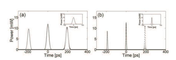
Fig. 4. Numerical traces of the pulses at the delay generator input (inset) and output for  $\Delta\omega=-1.5$  THz (dashed line),  $\Delta\omega=0$  (solid line) and  $\Delta\omega=1.5$  THz (circles) for : (a) 25-ps pulse width and 5-W pump and (b) 6.5-ps pulse width and 20-W pump power.
