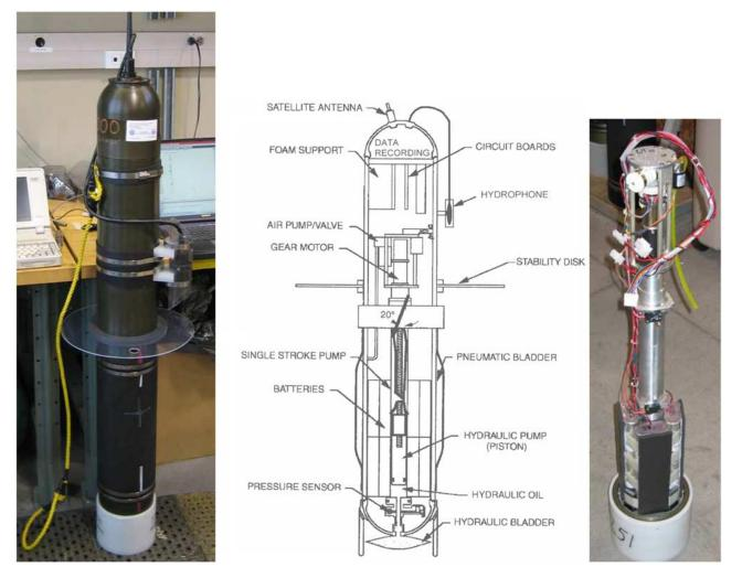
**Figure 1.** The MERMAID prototype: a SOLO float equipped with an externally mounted hydrophone and a recording and processing unit. (left) Outside view. (middle) Design schematic. (right) The interior rise-and-dive mechanism, cabling, and lithium battery packs.
