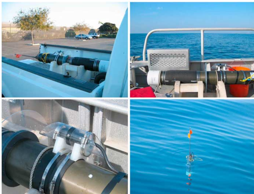
Figure 2. Scenes from the MERMAID deployments in the waters offshore San Diego, CA. (top) Transportation to and from the deployment location by truck and boat. The secondary bladder, a rubber sleeve filled with air, is seen in a semi-inflated condition. (bottom left) Close-up of the side-mounted hydrophone. (bottom right) Surfacing between dives, with the ARGOS satellite antenna emerging.
