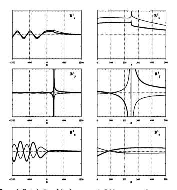
Figure 4. Perturbation of the three magnetic field components for a wave of class 3 (thick line=real part, thin line=imaginary part). The zone of the singularity is enlarged in RHS column.
