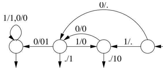
FIGURE 6. The successor function for the Fibonacci system.
