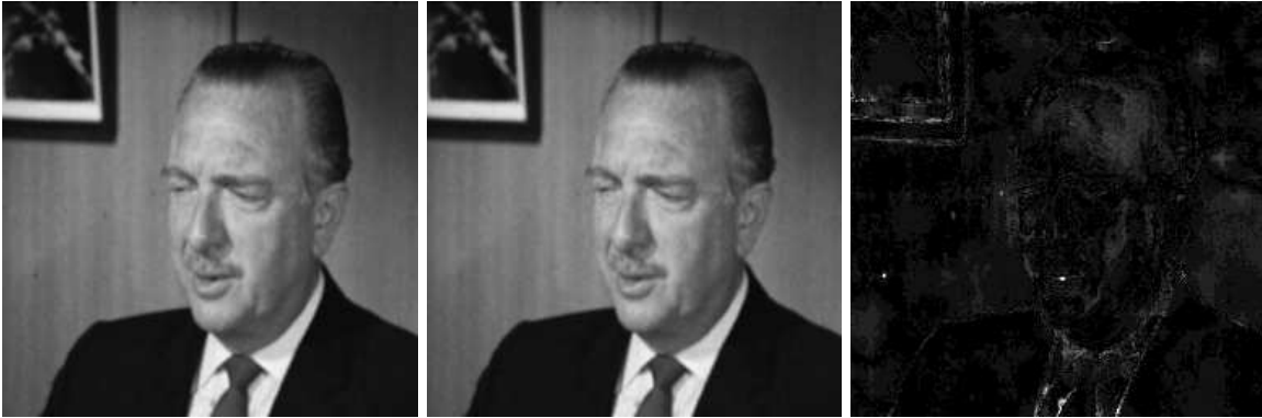
FIG. 4.1. Left: a frame of a sequence containing no visible flicker. Center: same frame, after applying Equation (3.3) with h = 10 to the whole sequence. Right: difference between both frames, rescaled from [0, 15] to [0, 255] for better visualization.
