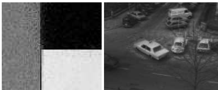
FIG. 4.5. Left : center of a frame of the flag sequence with the random local flicker, after a local stabilization by WP , with h = 30 . For this value of h , some artefacts appear around the singular zones (here the area around the intersection between the three regions). Right : extract of a frame of the taxi sequence with the motion-coherent flicker, after a local stabilization by WP , with h = 100 . Observe the artefacts around the zones of motion.
