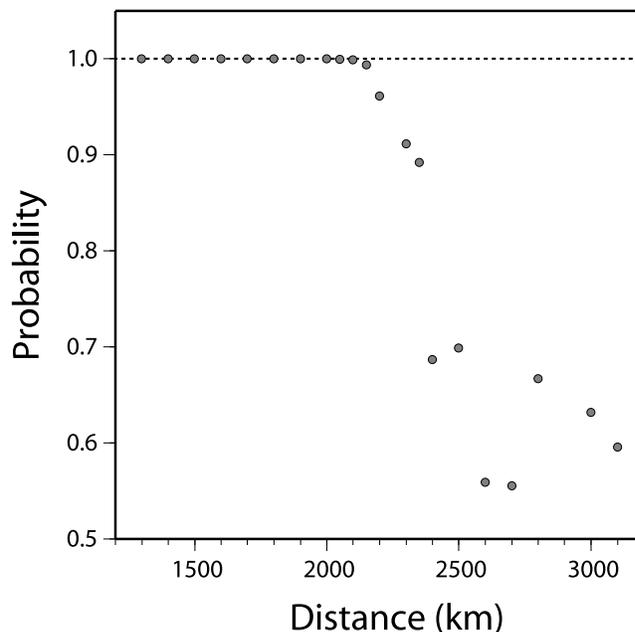
**Figure 7.** Improvement in fit to horizontal GPS velocities from the North American plate interior of a two subnetwork model relative to a single network model as a function of distance to the center of the GIA uplift. The probability of the observed improvement in the least squares fits of the two network model is determined using an F ratio test for 3 versus  $2N-3$  degrees of freedom, where  $N$  is the number of GPS sites (267) used for the comparison.
