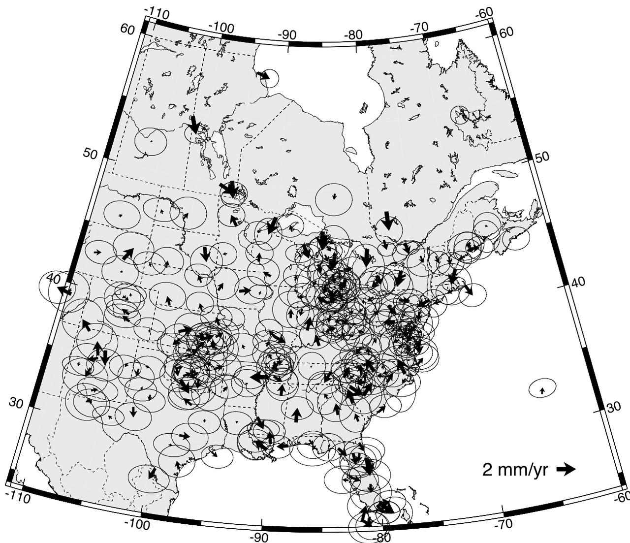
**Figure 12.** Residual velocities after removal of the best fit NOAM/ITRF2000 angular velocity. Only sites with velocity standard deviation less than 1 mm/yr and velocity magnitude less than 2.0 mm yr<sup>-1</sup> are shown here. Ellipses are 95% confidence.
