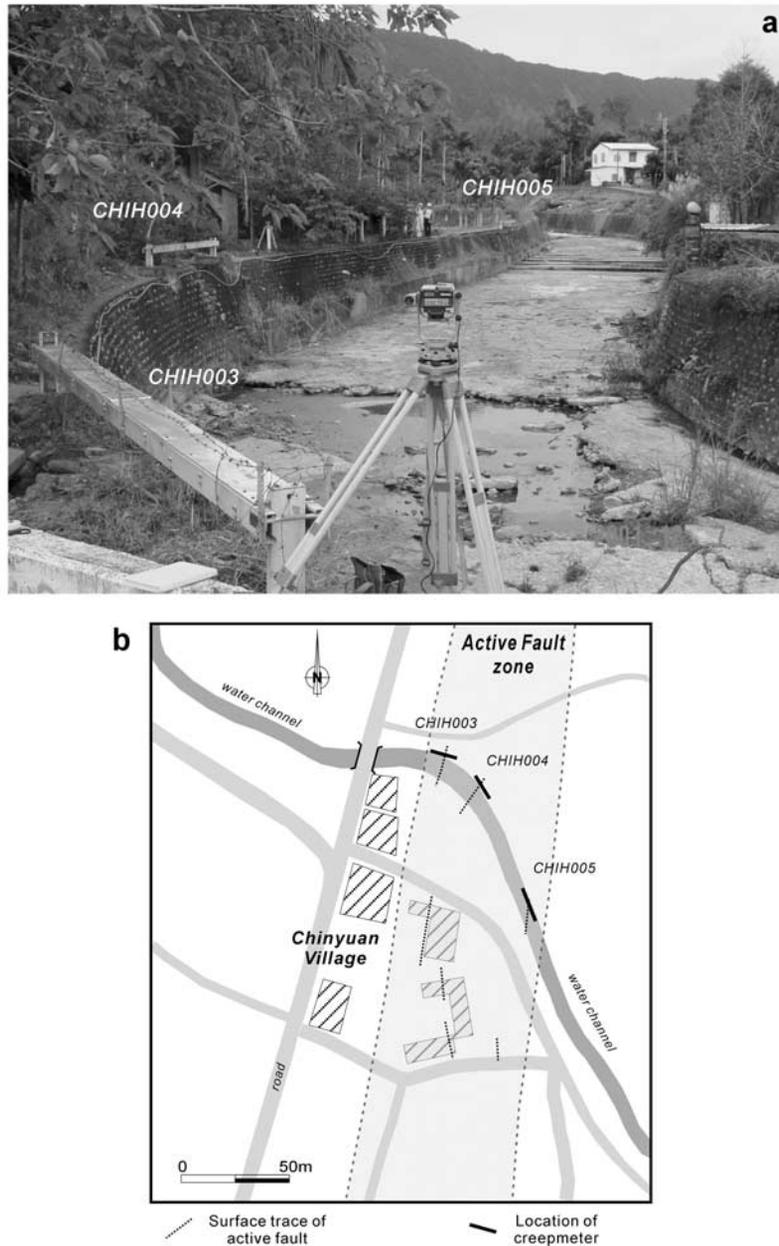
**Figure 7.** (a) Photograph and (b) location map of the creep meters at the Chinyuan site. Three creep meters (CHIH003, CHIH004, and CHIH005) were installed on the wall of the water channel where three surface ruptures of the active Chihshang Fault have been observed within about an 80-m-wide zone.
