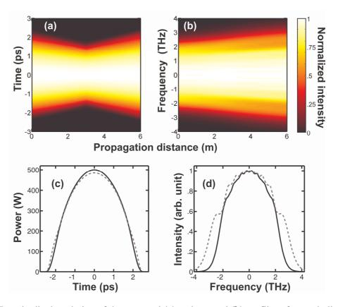
**Figure 2 :** Longitudinal evolution of the temporal (a) and spectral (b) profiles of a parabolic pulse in a set of two fibres (map1). Initial (solid line) and final (dashed line) temporal (c) and spectral (d) profiles are compared.
