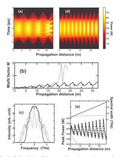
**Figure 3:** (a) Longitudinal evolution of the temporal intensity over 4 maps made of fibres 1 and 2 (b) Longitudinal evolution of the misfit parameter for map 1 (dashed grey line) and for map 2 (solid black line)
