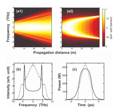
**Figure 4:** (a) Longitudinal spectral evolution over ten maps made of fibres 2 and 3 for an initial parabolic pulse (a1) and an initial sech pulse (a2). Comparison of the output spectral (b) and temporal profiles (c). Sech and parabolic pulses are plotted with solid black lines and dotted grey line respectively.
