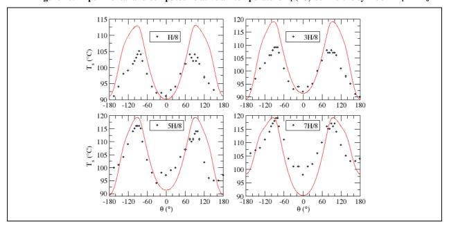
Figure 11: Experimental and computed cylinder temperatures for the reference test-case
