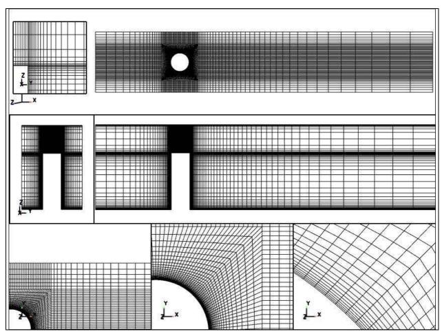
Figure 4: Meshing of the VALIDA test facility used for Code\_Saturne
