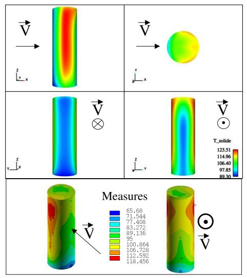
$Figure\ 7: Experimental\ and\ computed\ cylinder\ temperatures\ for\ the\ reference\ test-case$
