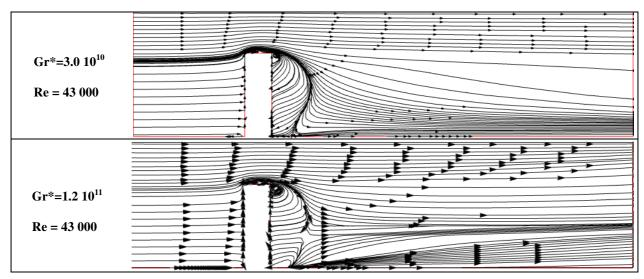
Figure 6: Air stream lines for Re = 43 000 and two different  $Gr^*$  numbers -  $Gr^*$ =3.0  $10^{10}$  and  $Gr^*$ =1.2  $10^{11}$
