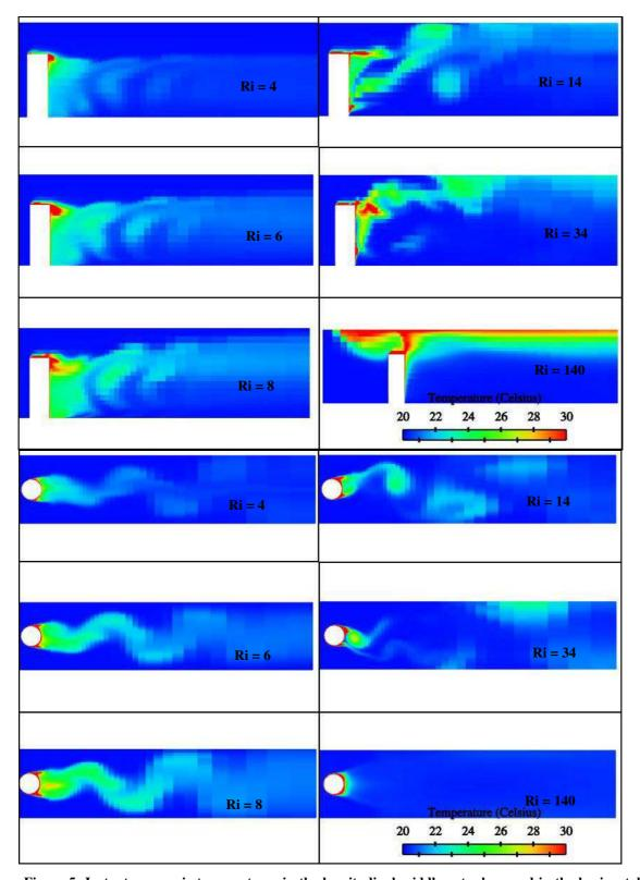
Figure 5: Instantaneous air temperatures in the longitudinal middle cut–plane and in the horizontal cut-plane at z=3H/2
