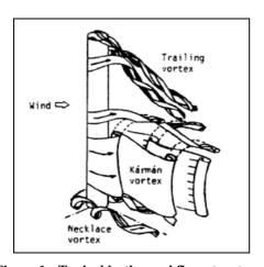
Figure 1: Typical isothermal flow structures
