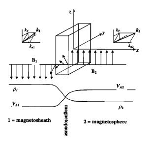
Figure 1. Equilibrium configuration of the model. The variations of the density and the Alfven velocity are superimposed to the geometrical sketch. The variation of the magnetic field direction is also sketched (for the case with a rotation).
