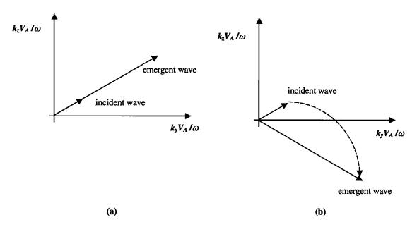
Figure 3. Evolution of the projection of the wave vector in  $(k_y V_A/\omega, k_z V_A/\omega)$  plane as the wave crosses the magnetopause layer: (a) without rotation of the magnetic field and (b) with rotation of the magnetic field.
