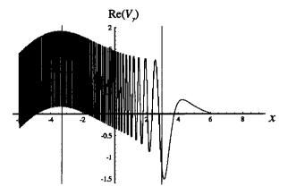
Figure 4. Solution without rotation. The quantity plotted is the real part of the  $v_y$  component of the velocity (y is the tangential direction perpendicular to B). The two dashed lines crudely indicate the limits of the magnetopause gradient (thickness of  $\sim 600$  km).
