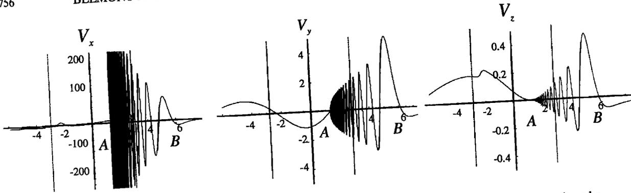
Figure 6. Solution with rotation. The three components of the velocity are plotted in a rotating frame (y and z rotate with the magnetic field). A and B refer to the points where (a)  $k_{||} = 0$  and where (b) the Alfvén mode becomes evanescent.
