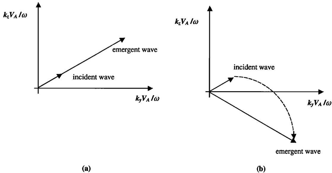
**Figure 3.** Evolution of the projection of the wave vector in  $(k_y V_A / \omega, k_z V_A / \omega)$  plane as the wave crosses the magnetopause layer: (a) without rotation of the magnetic field and (b) with rotation of the magnetic field.
