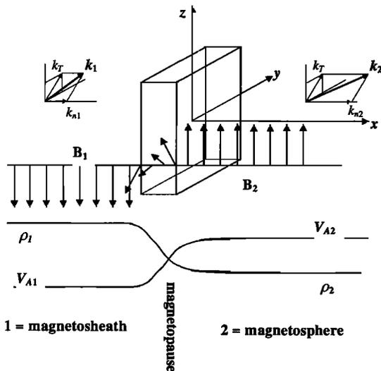
**Figure 1.** Equilibrium configuration of the model. The variations of the density and the Alfvén velocity are superimposed to the geometrical sketch. The variation of the magnetic field direction is also sketched (for the case with a rotation).
