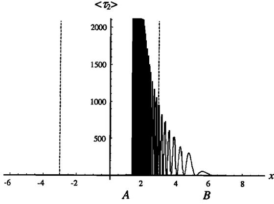
**Figure 8.** Reconnection rate in the  $x$  (normal) direction, calculated for the solution with rotation (Figure 6). The result evidences the localization of the reconnection phenomenon, but the numerical values (in  $\omega_c$  unit) can be disregarded.
