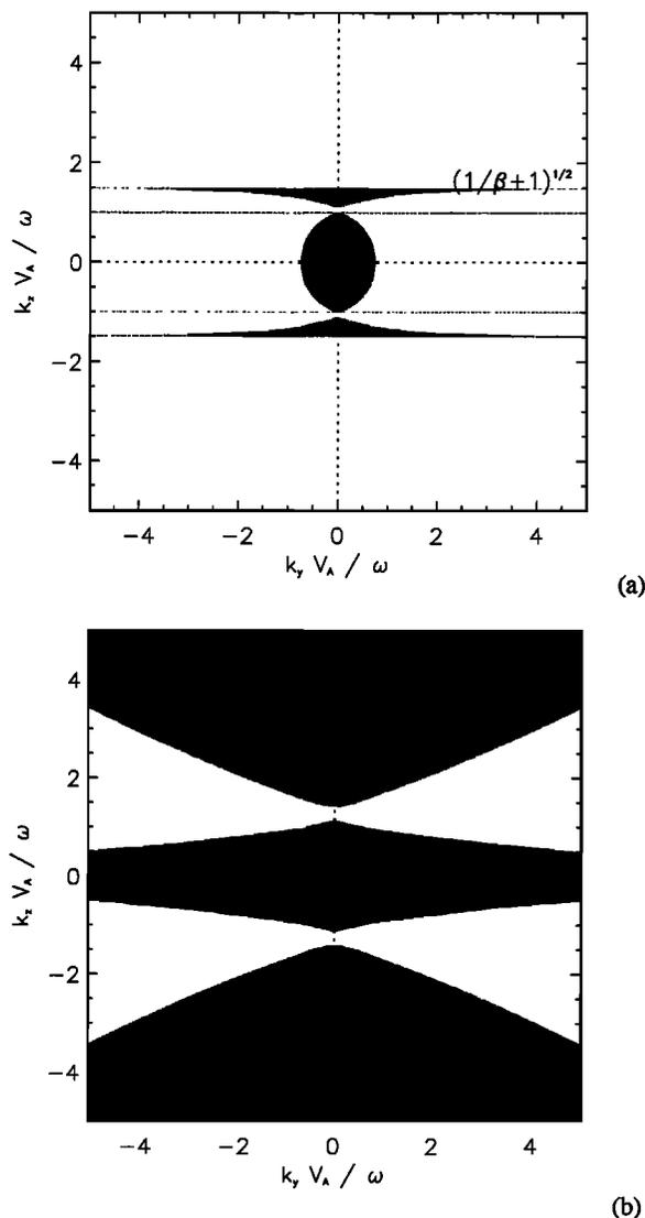
**Figure 2.** Projection of the dispersion relation in the  $(k_y V_A/\omega, k_z V_A/\omega)$  plane for two cases: (a)  $\alpha=0$  and  $\beta=0.8$  and (b)  $\alpha=0.5$  and  $\beta=0.8$ . The white regions of the plane correspond to cases where no propagating mode exist (all waves are evanescent), the gray regions correspond to cases where one mode can propagate and the black regions to cases where two modes can propagate.
