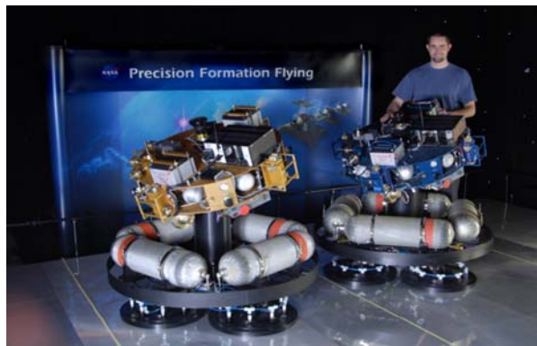
Fig. 10 The two robots of the formation control testbed at JPL. Each robot carries a mobile instrument platform (shown tilted), as well as canisters of compressed air to float the robot on a polished metal floor. The testbed has completed its functional testing and should achieve operational testing in 2007
