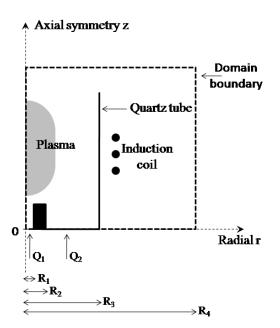
Figure 11: Schematic illustration of the plasma torch.
