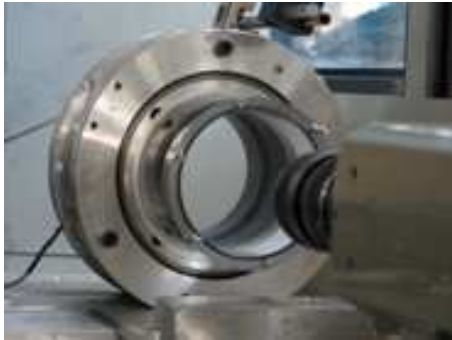
Figure 2: Photography of the experimental device showing the tank. In front of it is the high-speed camera. In the back the toothed belt and the opto-electronic sensor can be seen.
