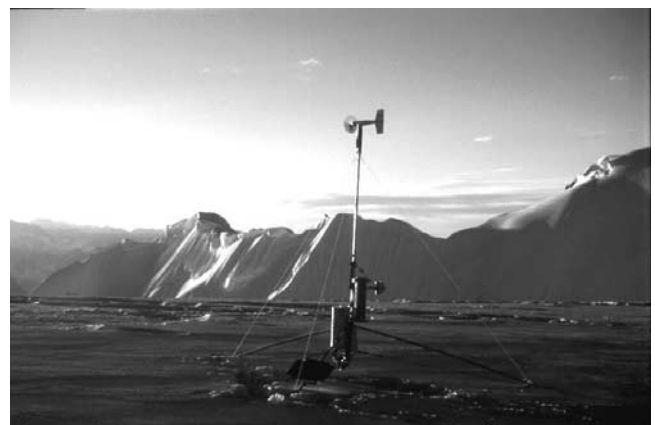
Figure 2. Picture of the AWS installed on the field site on Illimani at 6340 m asl (May 25, 2001). Photo: P. Wagon.
