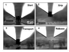
Figure 2: Teleoperated pick-and-place of a 40 µm micro-object
