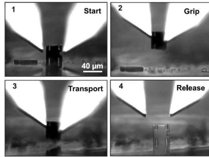
Figure 2: Teleoperated pick-and-place of a 40  $\mu\text{m}$  micro-object
