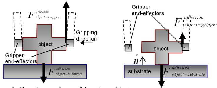
Figure 1: Grasping a release of the micro-object
