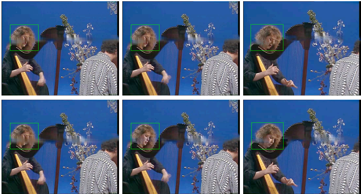
Fig. 9. From left to right: frames 97, 99 and 116 of Harp sequence. Top: Normal coding . Bottom: RoI coding 1 . The green box indicates the RoI.
