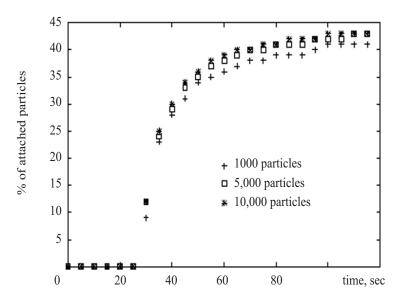
Fig. 6. Percentage of attached particles according to time (diameter =  $5 \mu m$ )
