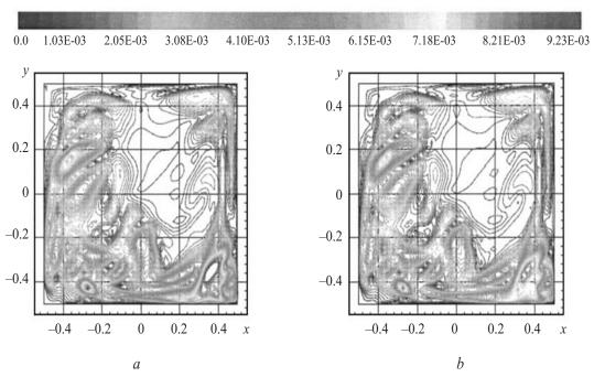
Fig. 5. Isocontours of fluctuating velocity magnitude at time t = 9 sec in the z = 0 plane: reference solution LES (a), obtained by solving DS (4 modes) (b)
