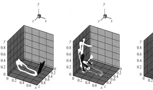
Fig. 7. Temporal evolution of the 5 μm particles' cloud in the cavity: Left: 20 sec (black), 64 sec (white); Right: 80 sec (black), 120 sec (white) since particles' injection
