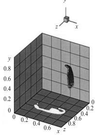
Fig. 8. Temporal evolution of the 10 μm particles' cloud in the cavity: 20 sec (black), 64 sec (white) since particles' injection)
