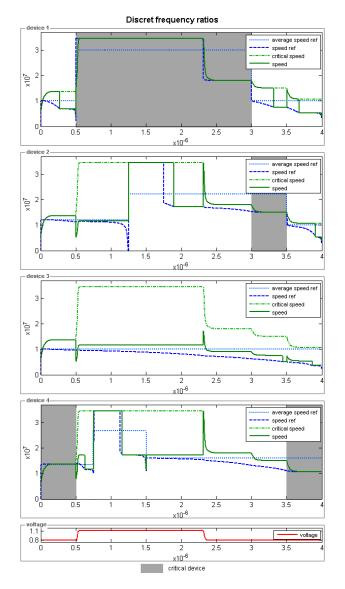
Fig. 9. Simulation results of the multicore controller based on partial duplication of the monocore control strategy (with discrete frequency ratios): energy consumption of  $4\cdot 10^{-5}J$  and computational needs of  $4.3\cdot 10^{5}flops$ , that is an increase of 1% of energy consumption and 11% of computational needs compared to the controller with *ideal* continuous frequency ratios
