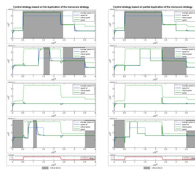
Fig. 7. Simulation results of the multicore controller based on full duplication of the monocore control strategy (with ideal continuous frequency ratios): energy consumption of  $3.976 \cdot 10^{-5}J$  and computational needs of  $5.8 \cdot 10^5 flops$ , that is 82.2% of energy consumption and 94% of computational needs compared to a controller without DVS
