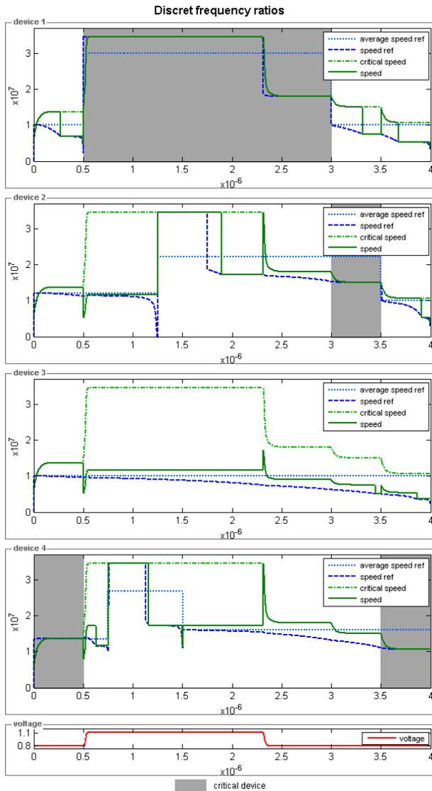
Fig. 9. Simulation results of the multicore controller based on partial duplication of the monocore control strategy (with discrete frequency ratios): energy consumption of  $4 \cdot 10^{-5} J$  and computational needs of  $4.3 \cdot 10^5 fops$ , that is an increase of 1% of energy consumption and 11% of computational needs compared to the controller with *ideal* continuous frequency ratios
