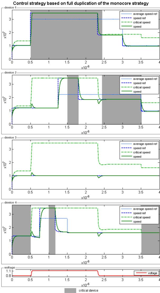
Fig. 7. Simulation results of the multicore controller based on full duplication of the monocore control strategy (with *ideal* continuous frequency ratios): energy consumption of  $3.976 \cdot 10^{-5} J$  and computational needs of  $5.8 \cdot 10^5 fops$ , that is 82.2% of energy consumption and 94% of computational needs compared to a controller without DVS
