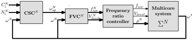
Fig. 4. Multicore control architecture based on full duplication of the monocore control strategy: the *computational speed controller (CSC)* and the *frequency and voltage level controller (FVC)* are duplicated as much as devices and a *frequency ratio controller* calculates the critical frequency and voltage level to deduce the frequency ratios  $\rho^N$ .
