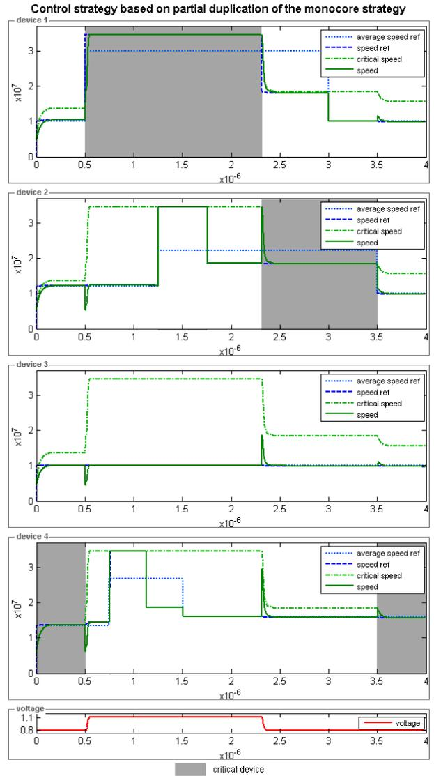
Fig. 8. Simulation results of the multicore controller based on partial duplication of the monocore control strategy (with *ideal* continuous frequency ratios): energy consumption of  $3.98 \cdot 10^{-5} J$  and computational needs of  $3.8 \cdot 10^5 fops$ , that is 82.4% of energy consumption and 62% of computational needs compared to a controller without DVS
