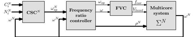
Fig. 5. Multicore control architecture based on partial duplication of the monocore control strategy: only the *computational speed controller (CSC)* is duplicated as much as devices and then a *frequency ratio controller* calculates the critical speed set point which will be used by the *frequency and voltage level controller (FVC)* and deduces the frequency ratios  $\rho^N$ .
