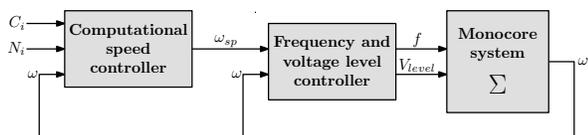
Fig. 2. Monocore controller architecture: a **computational speed controller (CSC)** plus a **frequency and voltage level controller (FVC)**
