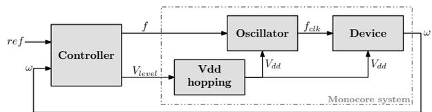
Fig. 1. Monocore system architecture
