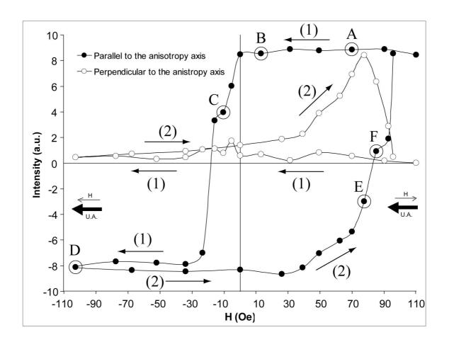
FIG. 2. Hysteresis loops calculated from whole set of magnetic maps for different *in-situ* applied fields. The solid lines are guides to the eye. Magnetic paths (1 and 2) described in the
