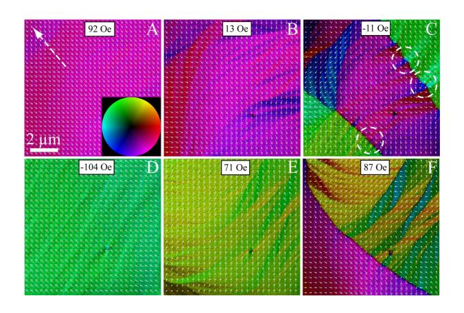
FIG. 1. 6 magnetic maps obtained by DPC on the Co<sub>35</sub>Fe<sub>65</sub>(70nm)/NiMn(50nm) bilayer. On the image (A) the unidirectional anisotropy direction is represented by the dashed white arrow. The inserted color wheel indicates the direction of magnetization by the color and the intensity corresponds to the strength of the magnetic signal. On the image (C) some cross-tie walls are surrounded.
