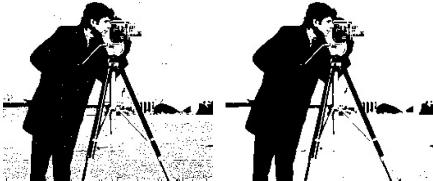
FIGURE 4. Segmentation of the cameraman image using L2 -fidelity (left) and L1 -fidelity (right), with the same weights ( \mu = 1 and \lambda = 0.1 )
