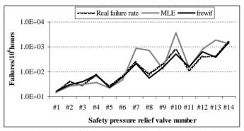
Figure 8. Results of failure rate evaluations using 3 times to failure observed per valve (logarithm scale)
