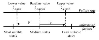
Figure 2. Fundamental assumptions of the proposed model
