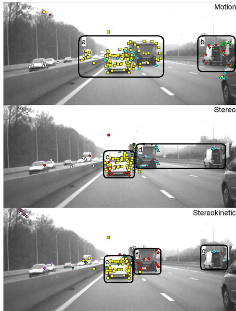
Fig. 6. Clustering results with motion based method (top), stereovision based method (middle), and stereokinetic based method (bottom)
