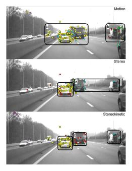
Fig. 6. Clustering results with motion based method (top), stereovision based method (middle), and stereokinetic based method (bottom)
