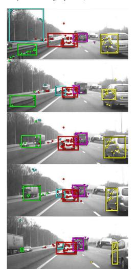
Fig. 5. Clustering results on a real sequence at different times
