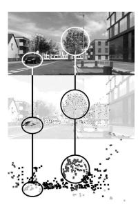
Fig. 3. Sparse optical flow and disparity map (light points are near to the camera and dark points are far) on a virtual sequence
