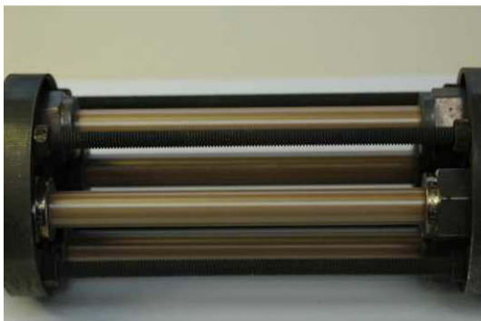
Fig. 1. Sample holder with four 12 cm-long oxidized claddings.
